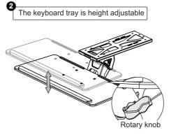
the lower right keyboard tray rotary knob in the lower right firer then adjust the tilt angle of the keyboard tray for using it in comfort, tighten the rotary knob after adjusting.
